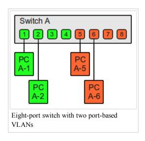
Although all of the PCs have been connected to one physical switch, only the following PCs can communicate with each other due to the configuration of the VLAN:
