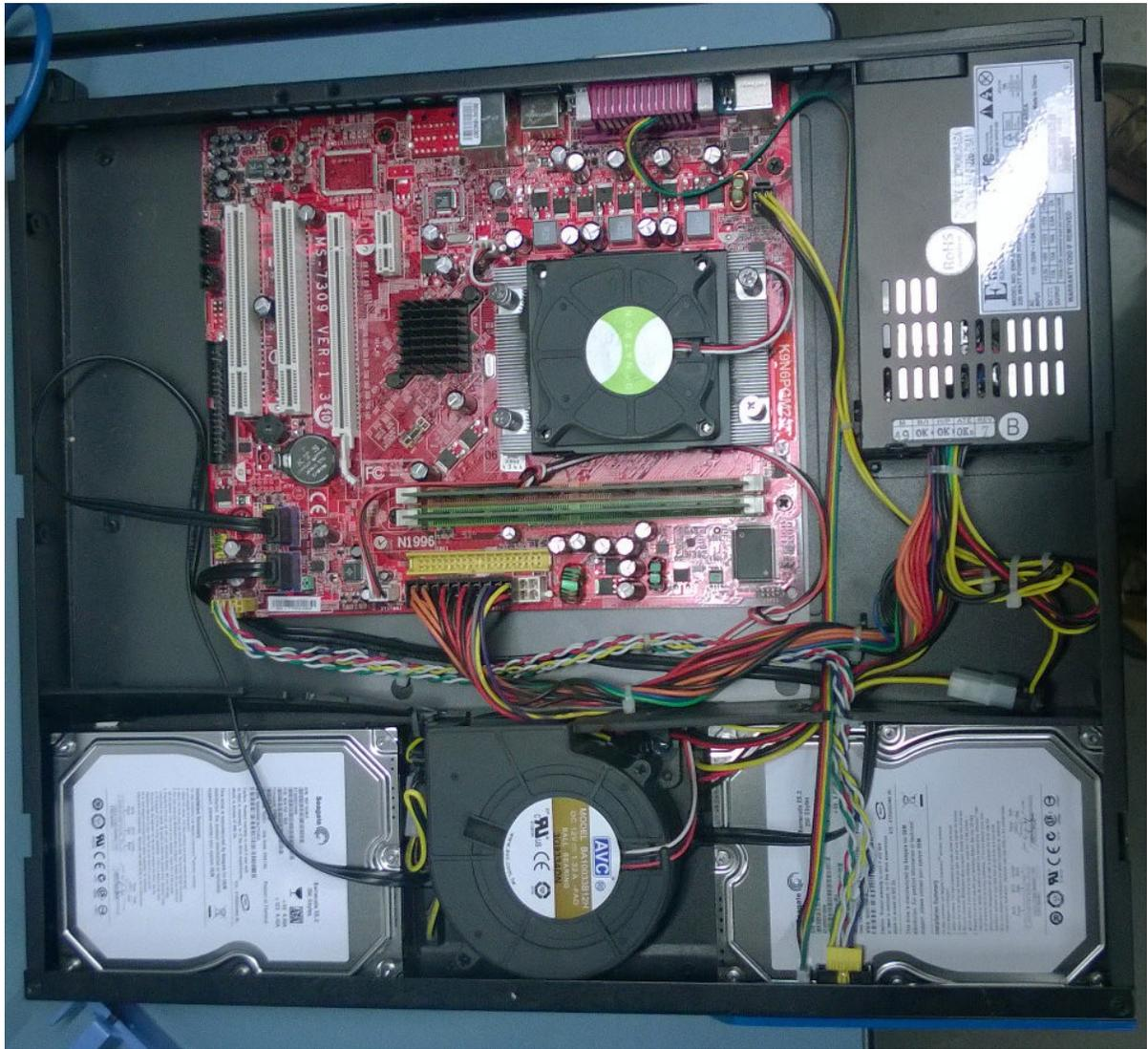
As you can see, the disks are partly covered by the lip of the front plate, some wiring, and are wedged in with black pieces of plastic. The black plastic pieces are glued onto the faring of that cooling fan in between the disks, but they are not glued at the other end.
